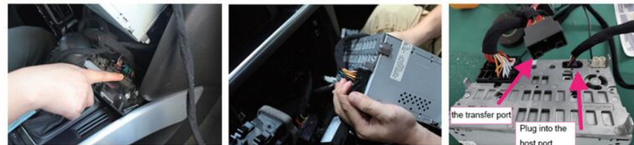
Complete the transfer of air conditioning panel
