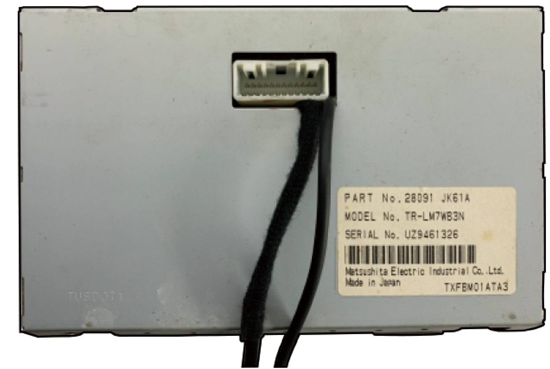
5, Finally assemble back the back cover, be aware of the VLDS and control cable outlet location
